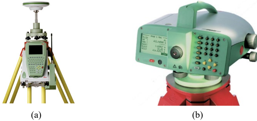
Figure 2. (a) Leica 1200 Differential GNSS Set-up (b) Leica DNA 03 Digital level
