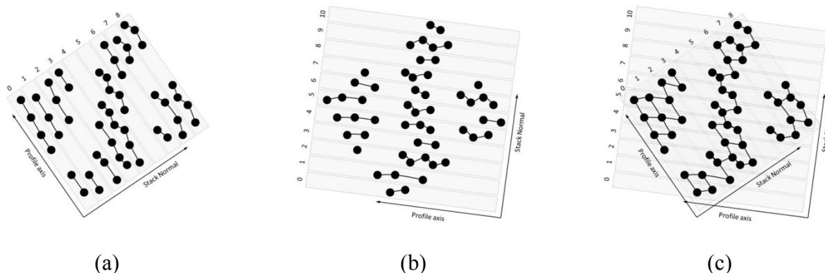
Figure 5. Segmentation of the point cloud. Segmentation of profiles in Stack 1 (a), Segmentation of profiles in Stack 2 (b) and Overlay of stacks 1 and 2 (c).
