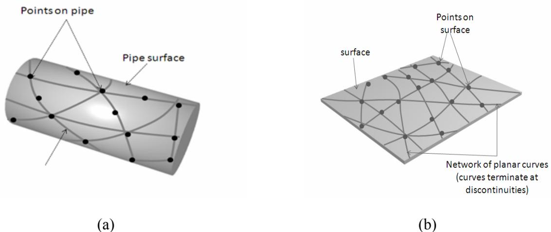
Figure 2. Network of planar curves representing a surface
