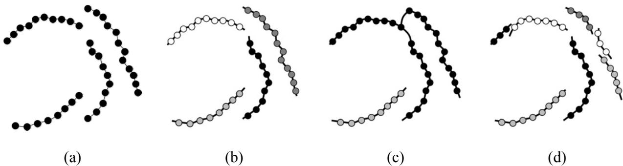
Figure 8. The choice of algorithm and parameters can yield a correct detection of the curves, a merging of the curves, or an over segmentation of the curves. (a) Points taken from a single profile in a stack. (b) ideal segmentation, (c) under segmentation, (d) over segmentation.
