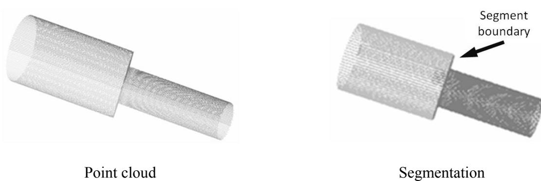
Figure 13. Segmentation of a coaxial pipe.
